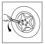
Loosen all plastic caps by turning the wheel wrench counterclockwise.
